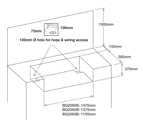
NOVA GRAPHITE SINK, BIN AND STORAGE MODULE PLUMBING DIMENSIONS MODEL NO: BQ2191
