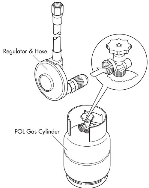
Screw the coupling nut of regulator into the cylinder valve outlet.
