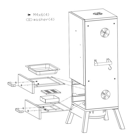
Locate the rack supports as required on each side of the smoker cabinet or alternatively adjust the top rack then utilise the hanging hooks.
