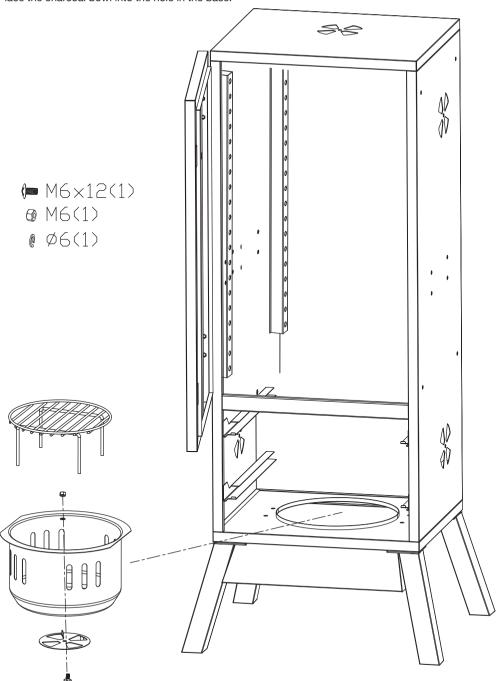
Attach the handles using eight M6x12mm screws and nuts. Attach the five rotating air vents as shown using five M6x12mm screws, washers and nuts, ensuring that they can be fully closed.
