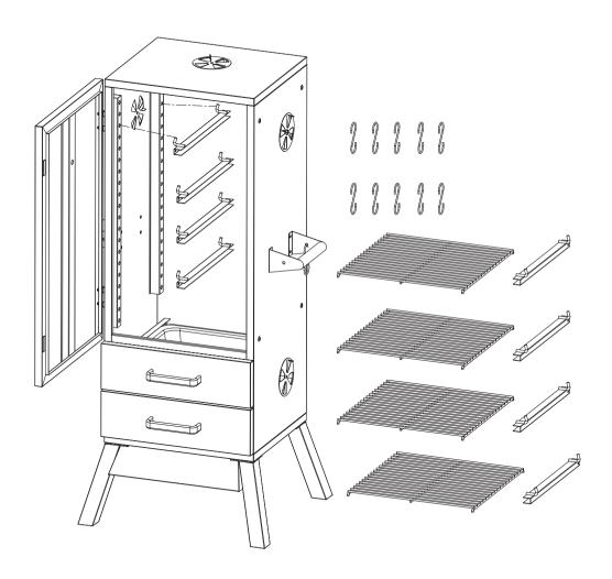
Attach the temperature gauge, bezel using the attached nut and the door handle using two M4x6mm screws and fibre washers.
