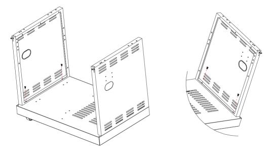
Use M6\*12 screw (x5pcs) to fix the back panel onto base panel, cabinet left side panel and cabinet right side panel.
