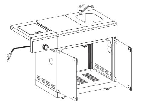
Remove the cylinder slide tray from BBQ and then attach it to the corresponding position inside the sink module's cabinet.
