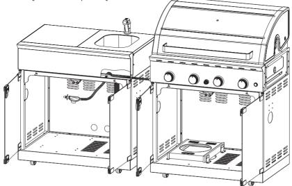
Use M6\*16 screw (x4pcs) and Flange M6 Nut (x4pcs) to connect the sink module to the left of BBQ.
