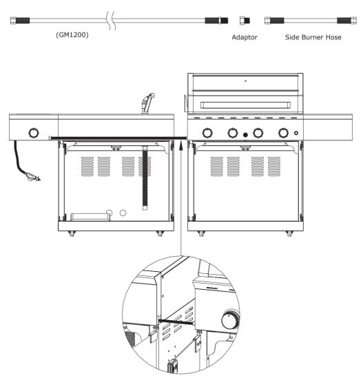
Use M6\*16 screw (x4pcs) and Flange M6 Nut (x4pcs) to connect the sink module to the left of BBQ.
