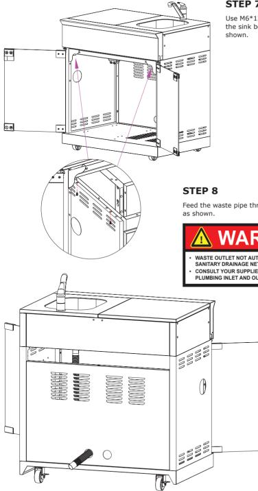
Use M6\*12 screw (x4pcs) to fasten the sink body assy to cabinet cart as
