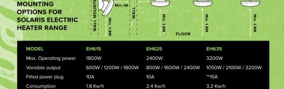
\*Note: Running costs based on an average tariff of \$0.49c/kWh. Check with your local energy retailer for confirmation. \*\*NOTE! MODEL 3200W REQUIRES A 15A POWER POINT TO BE INSTALLED BY A QUALIFIED ELECTRICIAN
