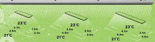
HEATING COVERAGE: THESE DIAGRAMS SHOW THE HEATING COVERAGE OF THE SOLARIS ELECTRIC HEATERS
