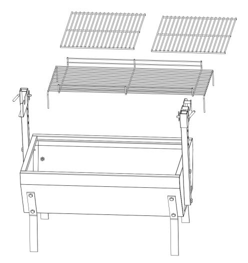
Slide the motor onto the support assembly, then position the prongs sleeve and handle onto the rotisserie shaft as required.
