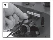
Check that the switch on the unit is in "OFF" position and then connect the power cable for the 12VDC Power Supply. Connect the male cigarette fitting to a suitable DC power source.
