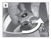
Turn the gas cylinder on in an anti-clockwise direction one (1) full turn, then check all LP Gas connections for leaks with a solution of soapy water (do not use a flame). If a leak is detected turn the cylinder valve off, allow any residual gas to disperse, retighten all connections then retest.
