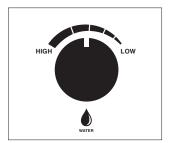
To increase Water Temperature turn GAS Control to MEDIUM / HIGH & allow temperature to stabilise. The Watertech Hot Water System is equipped with the following safety features:
