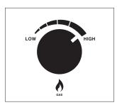
1. To increase Water Temperature turn GAS Control to HIGH and allow temperature to stabilise.
