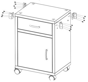
Attach four M6 screws and nuts to the upper holes of the side shelf brackets.
