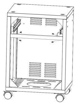
Attach the spring hinge pin to the door and attach the door handle using two M4 screws.
