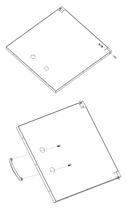
Attach the door to the cabinet with the spring hinge pin at the top and the solid pin at the bottom.
