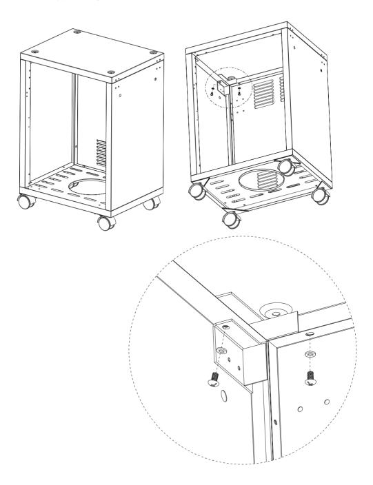
Attach the four strengthening brackets to the cabinet using sixteen M5 screws.
