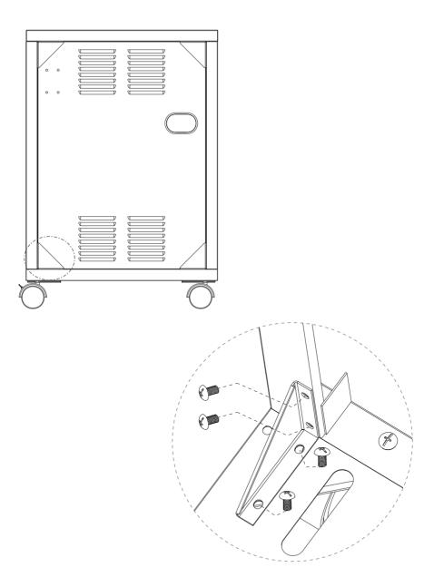
Attach the two drawer rail brackets to the side panels using eight M4 screws.
